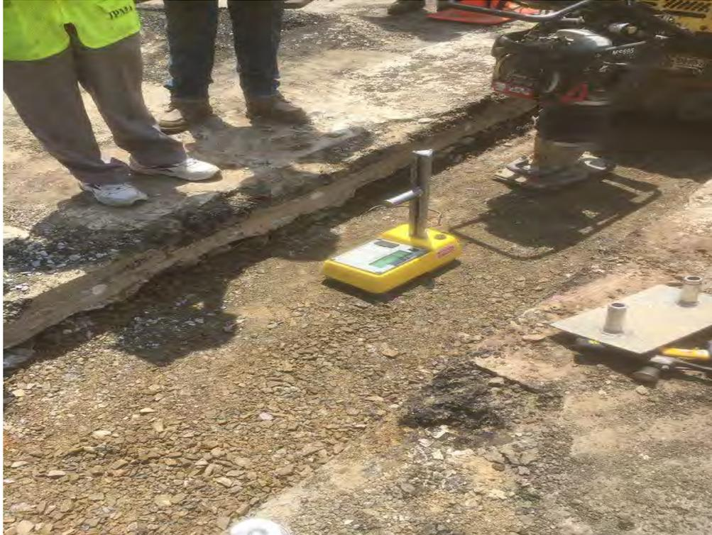
*Aggregate Base Compaction Testing before PCC Base placement*
