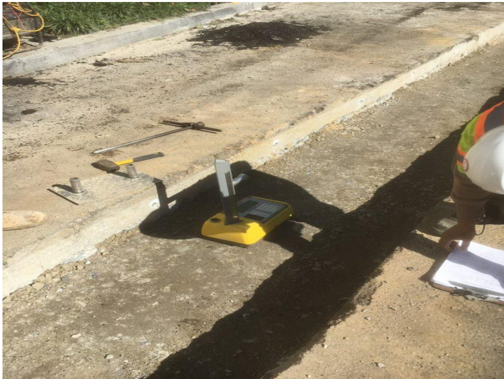
QA/QC compaction testing of Aggregate Base Material at 14 th and Florida Ave
