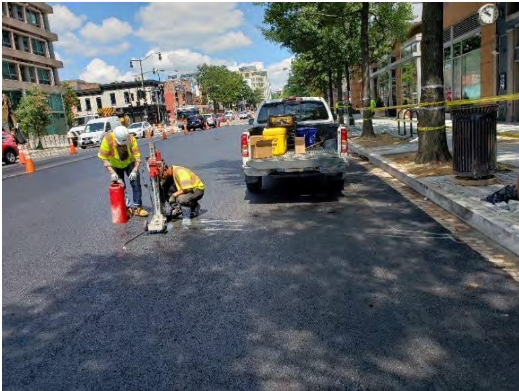
QC Techs cored 4 samples for Asphalt 12.5mm QC & Density Analysis at DC-d. Asphalt Lab
