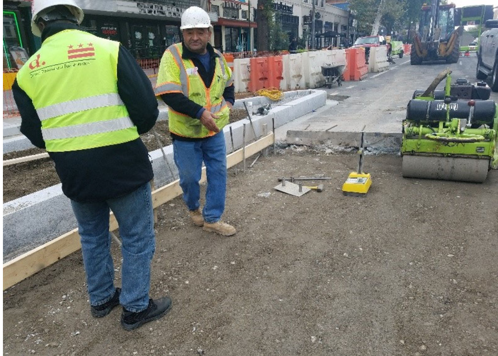
Density test of aggregate base course by DDOT operation.
